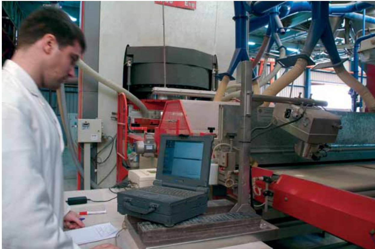
Automatic control system of a hydraulic press.
